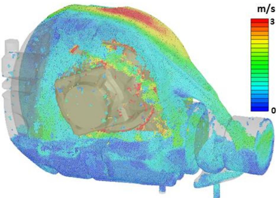
Liquid flow at a given moment. The MPS particle display color represents the absolute value of liquid velocity
